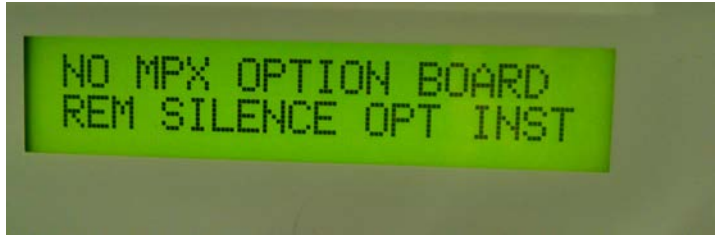
Fig. 3 Boot up Display message for a properly installed Alarm Status Board
