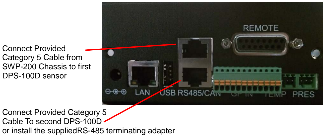
Fig. 1 Shows connection from SWP-200 Chassis and to succeeding DPS-100D Sensors or termination if only one sensor is supplied.
