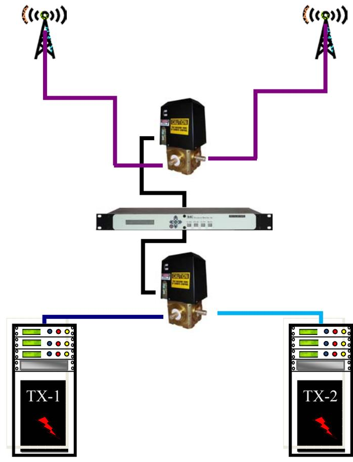
The SWP-200-2T series allows for a single rack unit solution to dual motorized switch control. This configuration allows for Main/Aux antenna selection and Main/Aux transmitter selection
