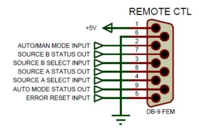
**Remote Control RS-232 Connection Diagram**
