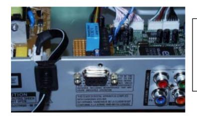
This photo shows the DB9 connector protruding from the rear panel. Make sure that whatever type of hole that you cut that you plan where the hole will be so that the connector doesn't interfere with the cover or components inside the player.
