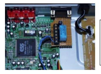
You can install the suggested circuit inside the player. Here we used a DB9 connector for connection and support. You can also use a 1/4" or 1/8" tip/ring/sleave phone jack. Use the tip and ring for connections and the sleave can be used for a ground between the player and CDS-302.
