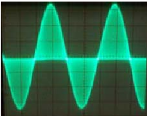
A properly adjusted L=-R gain adjustment 50 Hertz Left Only - Pilot has been removed
