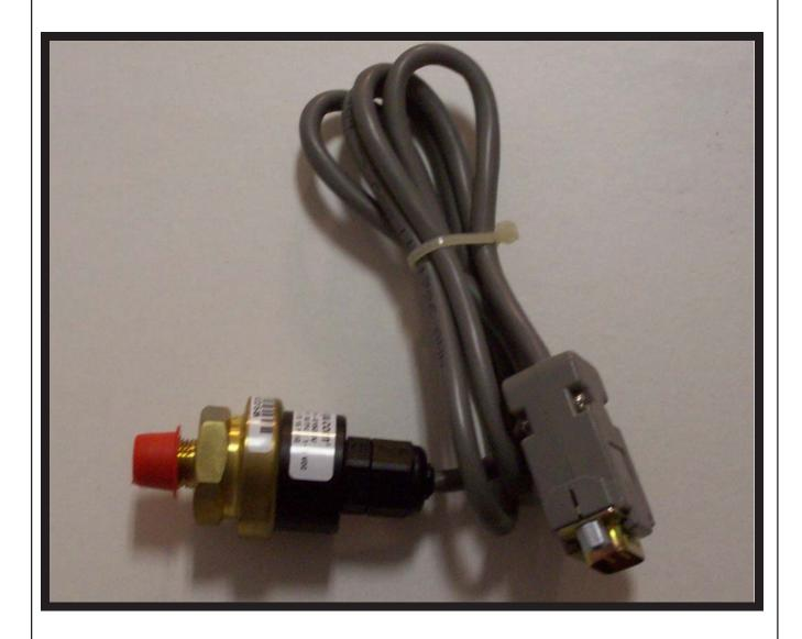
The PSW-100 is a 0-6 PSI pressure sensor. All power and data for operation is provided by the BDI SWP series chassis via a DB-9 connector.
