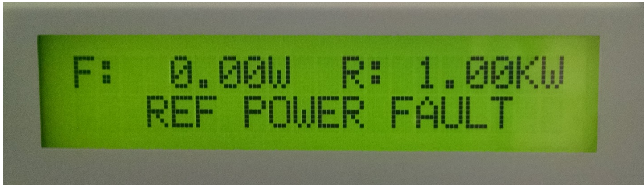
Fig. 4 Reflected Power Fault Indication
