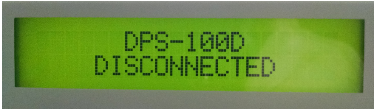
Fig. 1 RMD-100 Display showing DPS-100D Power Meter is disconnected
